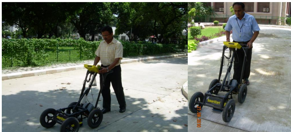
Figure 2a: 1000 MHz ground coupled antenna based GPR. Figure 2b: 1000 MHz GPR survey
